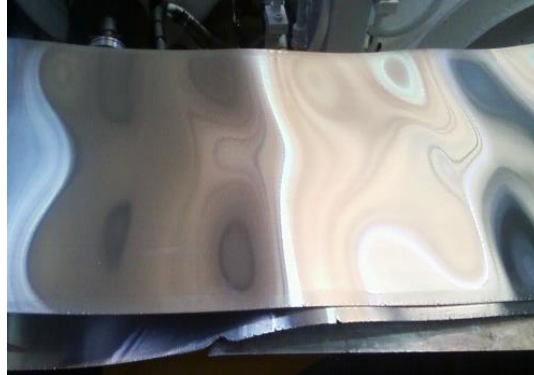
FIG. 25 View of flatness defects (wavy edges) generated by the cold rolling mill.
