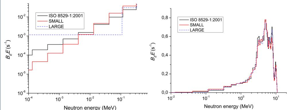
Fig. 2. <sup>241</sup>Am-Be spectrum: "small", "large" and "8529-1:2001".
