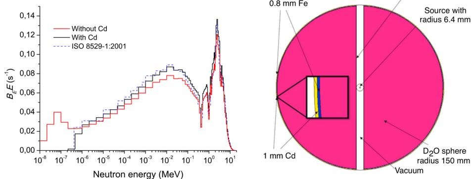
Fig. 1. <sup>252</sup>Cf(D<sub>2</sub>O) spectrum and construction.
