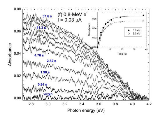
**Figure 3:** UV-visible absorption spectra of YSZ single crystal at RT: off-beam spectra after irradiation for various electron energies: 2.5 MeV (a, b), 1.75 MeV (c), 1.0 MeV (d), and 0.8 MeV (e), as a function of decay time. Solid lines are fits using Gaussian profiles. Insets: Decay curves versus time; solid and dashed curves are least-square fits with Eq. (2).
