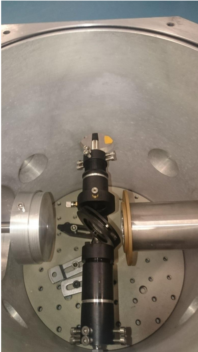
Figure 1: Picture of the experimental set-up: the electron beam entrance port of the irradiation chamber is on the left side with the diaphragm of 0.8 mm in diameter, the target sample is mounted at the center of the chamber at 45 deg. off-axis. The optical absorption measurements are carried out at 90 deg. off-axis.
