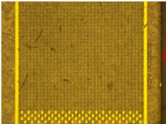
Figure 8. Photograph of the metallisation of the readout side. The bias column electrodes form a total of 1188 cells.
