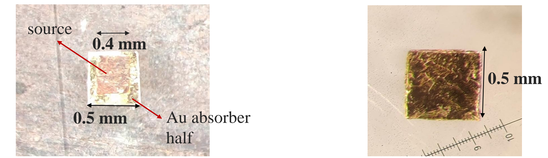
Figure 5: a) Source foil on one half of Au absorber b) Complete absorber-source ensemble.
