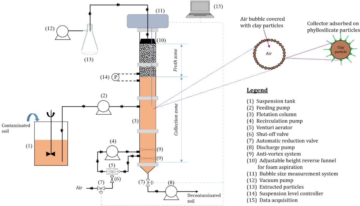
**Fig. 1.** Scheme of the continuous flotation experimental set-up.
