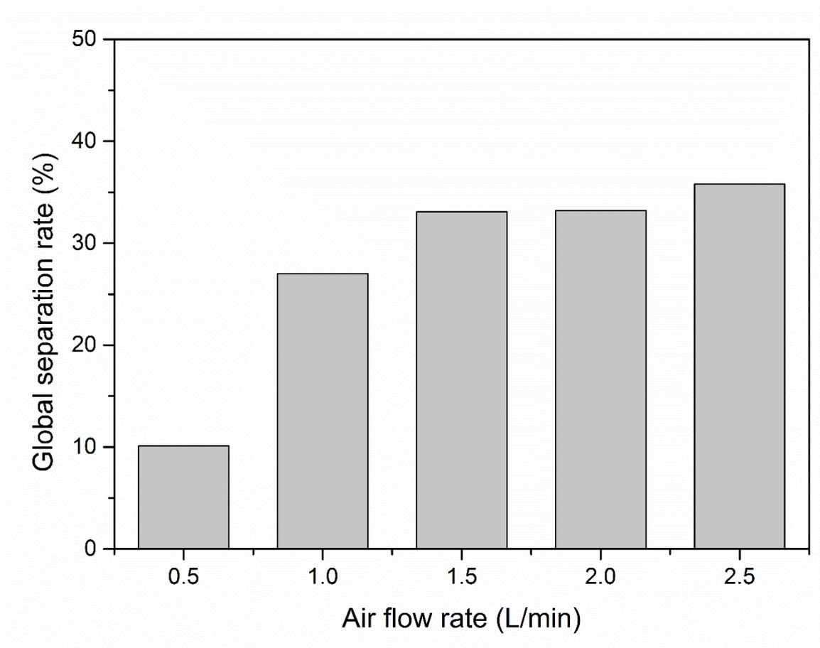
**Fig. 7.** Impact of air flow rate on the global separation rate at  $\tau=120$  s,  $C_s=50$  g/L and TTAB/soil ratio=0.2%.
