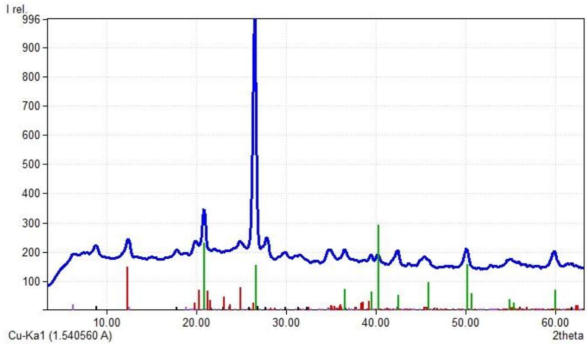
**Fig. B.** X-Ray Diffractogram of the 2-20  $\mu\text{m}$  froth particles separated from soil. Standards: quartz (green lines), illite (black lines), chlorite (violet lines), kaolinite (red lines).
