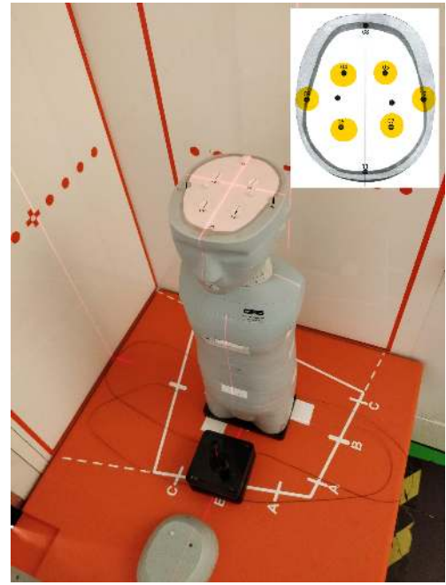
FIG. 1. Pediatric phantom set-up photo in the EOSedge. Phantom is in AP position. Upper slices of the phantom were removed to reveal the position of 6 OSL dosimeters in the brain. The corresponding hole index positions are shown on the schematic (top right).
