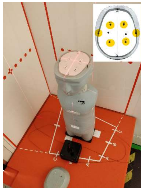
FIG. 1. Pediatric phantom set-up photo in the EOSedge. Phantom is in AP position. Upper slices of the phantom were removed to reveal the position of 6 OSL dosimeters in the brain. The corresponding hole index positions are shown on the schematic (top right).
