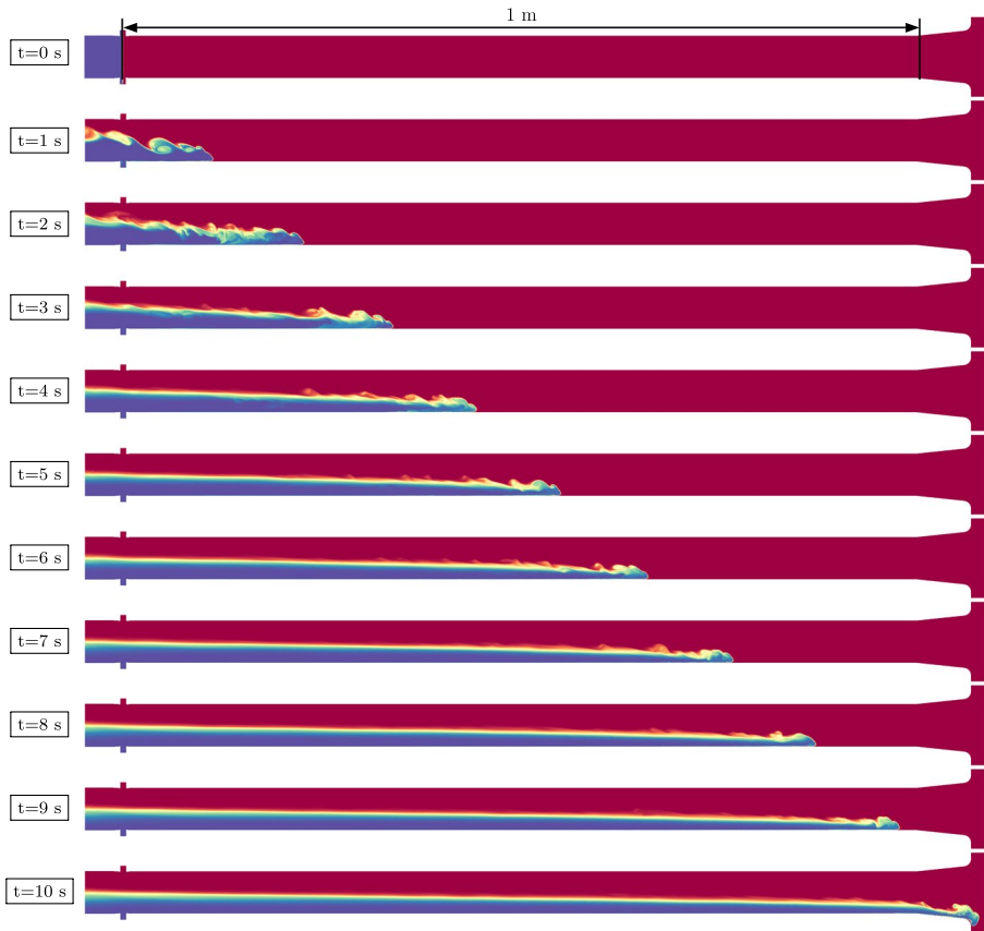
Fig. 7 Sequence of snapshots showing the evolution of the heavy fluid mass fraction in the cold leg obtained by the VD 4 simulation. The colour scale goes from 0 (red) to 1 (blue)
