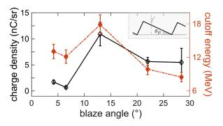
**FIG. 2.** Optimization of electron acceleration by using blazed gratings. <sup>15</sup> The total charge of the electron bunches and the cut-off energy in the detected spectrum are shown as a function of the blaze angle  $\theta_B$  (see inset for the definition). The resonant angle was 30° for the grating used, corresponding to  $d=2\lambda=1.6~\mu m$ . Adapted and partially reproduced with permission from Phys. Plasmas **25**, 031907 (2018). Copyright 2018 AIP Publishing.
