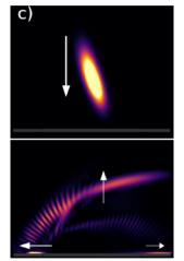
FIG. 6. Effect of the sign of wavefront rotation on surface plasmon generation. Two snapshots from Meep simulations at normal laser incidence on a grating are shown for (a) no rotation, (b) positive rotation, and (c) negative rotation. While in case (a) two symmetrical plasmons are generated, in cases (b) and (c) one plasmon is shorter and stronger than the other one. The parabolic-shaped signal is due to the scattering from the plasmon propagating along the grating.
