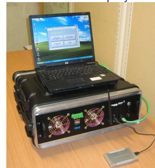
Opto-electronic module (19" - 3U) Laptop + External USB hard disk either Ethernet or Wifi
