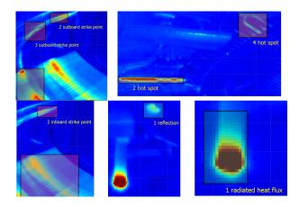
Figure 2. Examples of different hot spot annotations (from left to right: outboard strike point, hot spot, inboard strike point, reflection, radiated heat flux)
