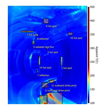
Figure 1. Annotation examples of several types of hot spots on the wideangle line of sight of the Tokamak WEST [4]
