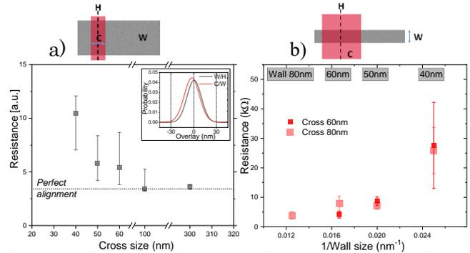
Fig. 4: a) Resistance (median values) measured wrt Cross size on dedicated test structures (PCM layer w/o OTS i.e. 1R devices) for alignment control. b) Evolution of mean  $R_V$  vs reciprocal of Wall size in 1R devices. The smallest Wall size of 40 nm shows a higher variability.
