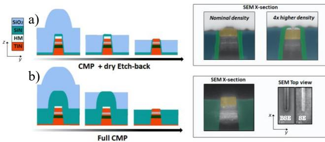
Fig. 3: Contact recovery after “Wall” patterning and encapsulation: a) “Etch-back” approach: strong dependency on the devices density. In the TEM it is compared the nominal (good) density wrt 4x (bad). b) “Full CMP” approach: good uniformity, confirmed by SEM (section + BSE and SE).
