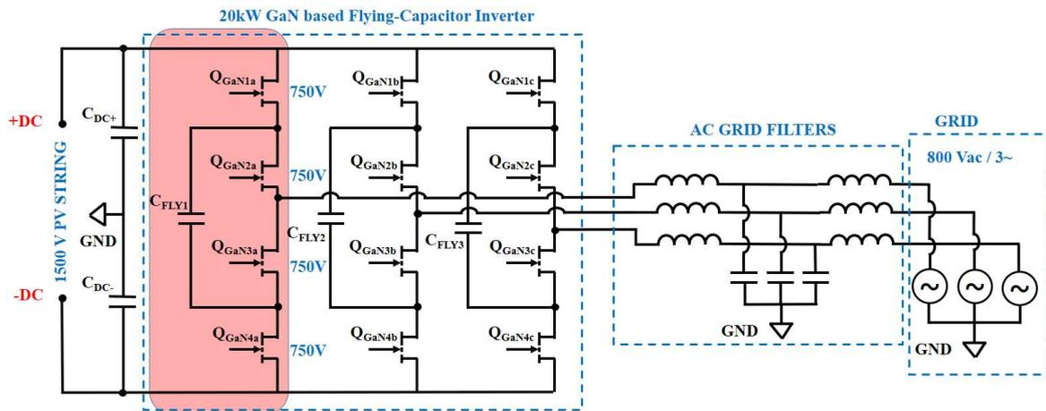
Fig. 14: Schematic of the 3-phase flying-capacitor inverter
