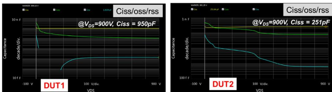
Fig. 1: Static characterizations of capacitances for GaN FET 900V (DUT1) and GaN HEMT 1200V (DUT2)
