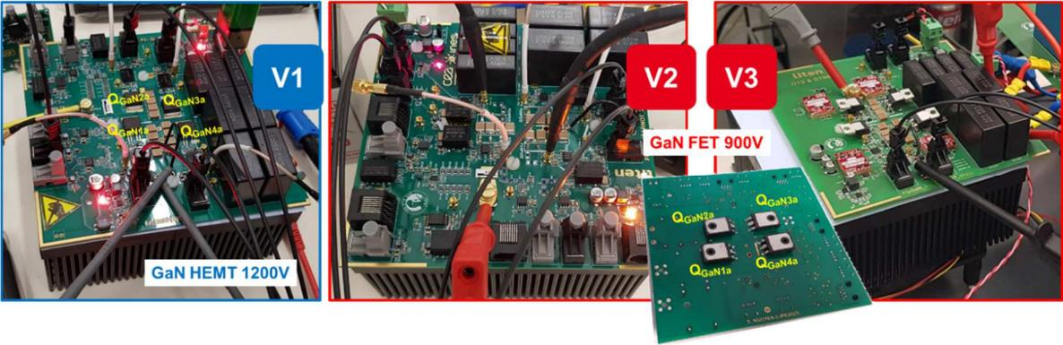
Fig. 15: Three different versions of GaN based active parts for the implementation of one-phase
