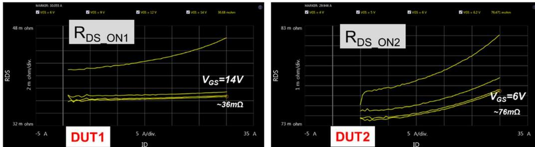
Fig. 3: Static resistances of GaN FET 900 V (DUT1) and GaN HEMT 1200 V (DUT2)
