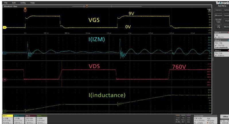
Fig. 6: Experimental waveforms of the DPT test
