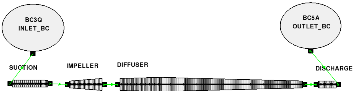
Fig. 2 : 1D-pump structure: four 1D elements (diffuser and volute belong to the same element)
