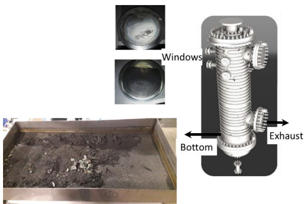
Figure 4. Residues collected at the bottom of the EFR, exhaust and on windows
