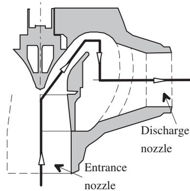
Figure 4: The hydraulic part of the pump (section)
