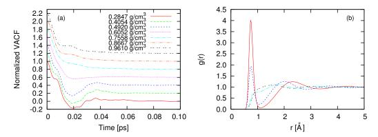
**Figure 1.** (Colour online) Non-monotonous density dependence of velocity autocorrelation functions (VACFs) in hydrogen fluid at T = 2500 K (a) and pair distribution functions for four densities (b). For convenience, the VACFs in (a) were shifted vertically with the step 0.2. Different lines in (b) correspond to the same densities as in (a).
