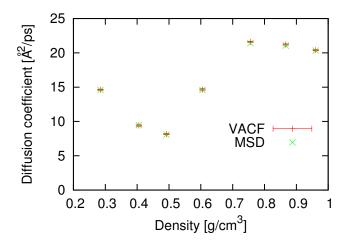
**Figure 3.** (Colour online) Non-monotonous density dependence of diffusion coefficients for hydrogen fluid at  $T = 2500 \, \text{K}$  and different densities, calculated from the velocity autocorrelation functions (shown in figure 1) by Kubo integral (plus symbols with error bars). A check of the diffusion coefficients via long-time asymptotes of the mean square displacements (cross symbols) shows very similar results.
