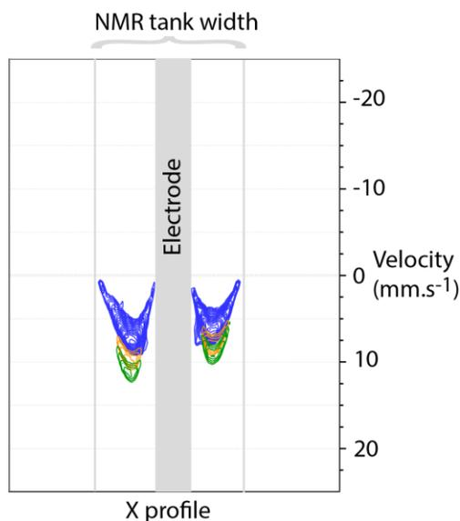
**Figure 4.** Velocity profiles of the solution inside the NMR tank, with a nitrogen flow of 1 mL/min (blue), 2 mL/min (orange) and 3 mL/min (green).
