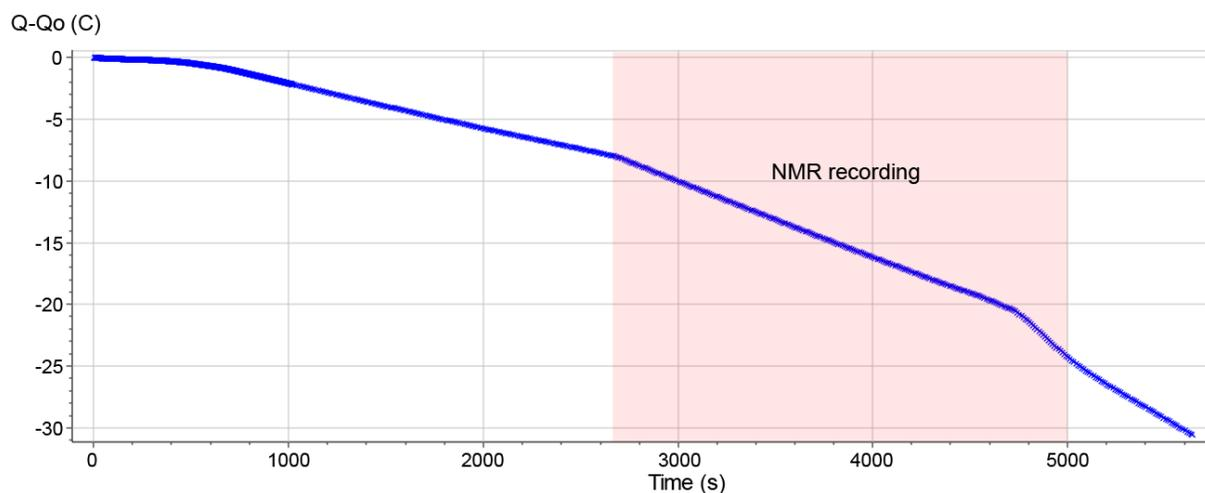
**Figure S11.** Chronoamperometry performed on the cell filled with oxidized 2,7-AQDS 50 mM in H<sub>2</sub>SO<sub>4</sub> 0.5 M (with solution flow). The time period in which the <sup>1</sup>H spectra have been recorded is represented by a pink area. The respective voltages applied are -0.3 V until the NMR starts (without effect on the anthraquinone; the first 1H NMR spectra still show the oxidized form) and -0.5 V after.
