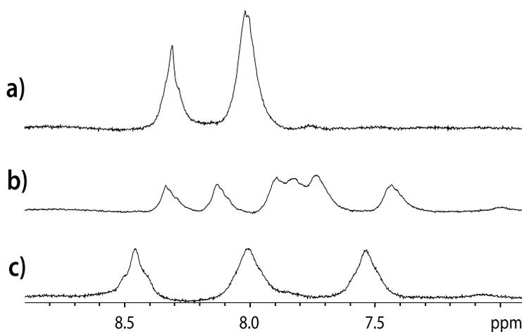
**Figure 5.** Three <sup>1</sup>H spectra of 2,7-AQDS during a reduction process. a) Oxidized form; b) Intermediate form; c) Reduced form.
