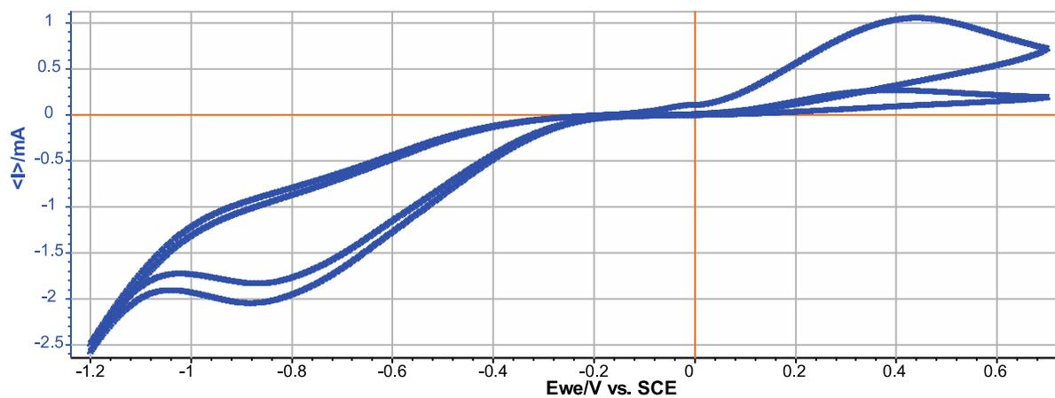
**Figure S10.** Influence of the magneto-hydrodynamic effect on the cyclic voltammetry. a) cell in a magnetic field lower than 5 gauss; b) cell placed inside the 11.7 T magnet. 2,7-AQDS 50 mM in  $\text{H}_2\text{SO}_4$  0.2 M without solution flow, scan rate 50 mV/s.
