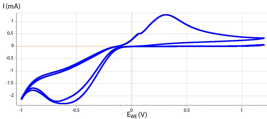
**Figure S9.** Cyclic Voltammetry recorded on the cell filled with oxidized 2,7-AQDS 50 mM in H<sub>2</sub>SO<sub>4</sub> 0.2 M (without solution flow). Scan rate 50 mV/s from +1.2 V to -1 V with 2 loops.
