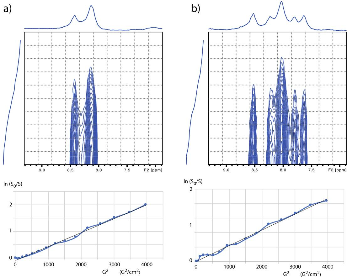
**Figure S13.** 2D DOSY experiments performed on a) the oxidized state of AQDS, b) the intermediate state where six  $^1H$  signals appear. At the bottom the curves  $\ln(S_0/S) = f(G^2)$  that have enabled extraction of the diffusion coefficients ( $S_0$  is the signal recorded with the lowest gradient value of 2.8 G/cm) are displayed. Note that the sum of all the aromatic proton signals has been used.
