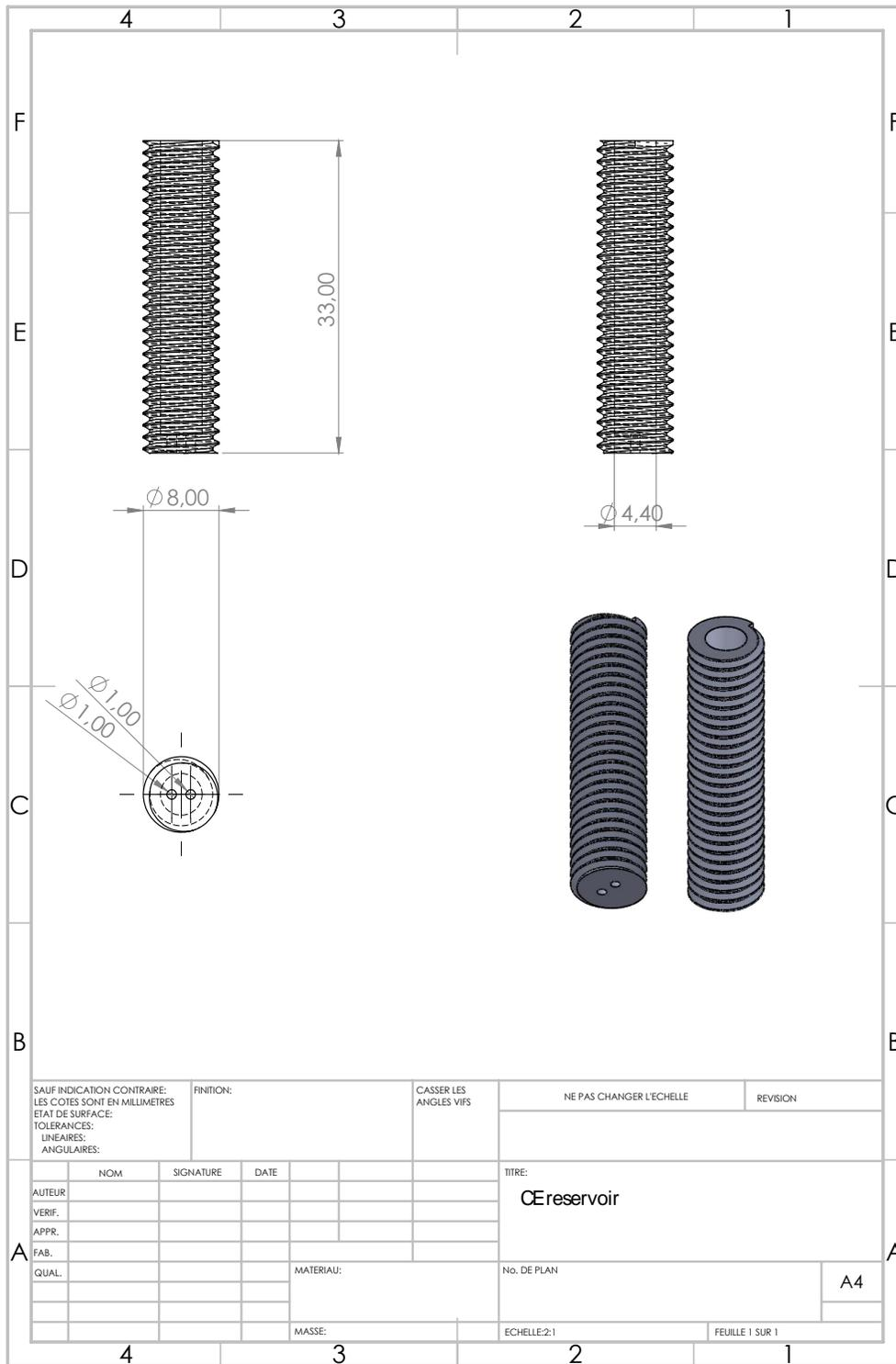
**Figure S6.** Drawing of the counter-electrode reservoir, to be inserted to the top part of the mini redox-flow battery. The Nafion membrane is stuck between these two pieces. The dimensions are in millimeters.
