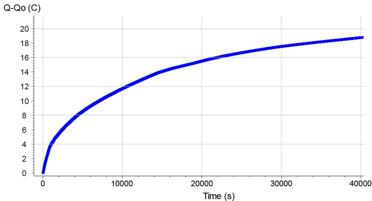
**Figure S12.** Chronoamperometry performed on the cell filled with reduced 2,7-AQDS 50 mM in H<sub>2</sub>SO<sub>4</sub> 0.5 M (with solution flow). A voltage of +0.45 V is applied.
