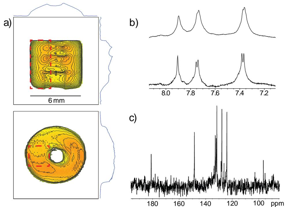
**Figure 2.** a) 2D  $^1\text{H}$  gradient echo images of the NMR reservoir. The presence of the electrode is clearly visible. b) Comparison between normal (4 scans, up) and localized (8 scans, down)  $^1\text{H}$  spectra of 2,7-AQDS (0.5 M). The selected area corresponds to the region delimited by the red dashed lines in a). c)  $^1\text{H}$ -decoupled  $^{13}\text{C}$  spectrum of 2,7-AQDS (0.5 M; 128 scans).
