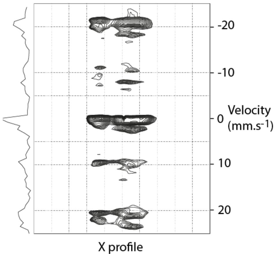
**Figure S8.** NMR velocimetry experiment performed with insufficient solution level inside the upper part of the insert. Signals on both sides of the zero frequency in the indirect dimension indicate that the solution oscillates but does not experience a net displacement.
