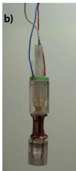
Figure 1. The mini redox-flow battery. a) Schematic diagram. WE: working electrode; RE: reference electrode; CE: counter-electrode. b) Picture; c) 3D rendering of the bottom (1), middle (2) and top (3) parts of the device. (4) Solution circuit loop, (5) NMR area, (6) back channel, rf-isolated with aluminum foil, (7) proton-exchange membrane, (8) counter-electrode compartment, (9) nitrogen inlet, (10) nitrogen exhaust, WE: working electrode (glassy carbon), RE: reference electrode (Ag/AgCl), CE: counter-electrode (Pt). For the sake of clarity, neither the rf coils nor the copper connectors at the bottom of the part (1) for the electric connection to the NMR probehead are drawn.
