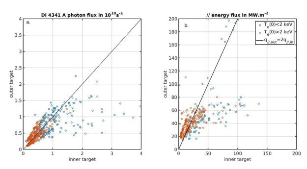
Figure 20. WEST C4–C5 L-mode database, B = 3.7 T,  $I_p = 0.5$  MA, LSN, D only,  $P_{tot} > 2$  MW. (a) shows the Dy photon flux: inner vs outer targets. (b) show the parallel heat flux on the outer target against the inner target flux.
