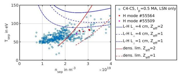
**Figure 19.** Separatrix operational space of WEST in terms of electron density and temperature. The red line shows the boundary of the L-mode density limit (equation (3) of [31]). The blue line indicates the L-H-L transition (equation (8) of [31]). The impact of  $L_{\perp}$  and  $Z_{\text{eff}}$  are tested: full versus dashed and dot-dashed lines. The H-mode phases are highlighted in red and magenta.
