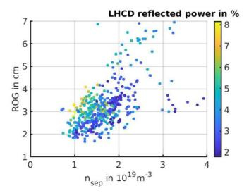
**Figure 15.** WEST C4–C5 L-mode database, B = 3.7 T,  $I_p = 0.5$  MA, LSN, D only,  $P_{\text{tot}} > 2$  MW. Color bar is the averaged LHCD reflected power in % (aveaged on the upper and lower rows of two LHCD launchers), time averaged over the plateaus.
