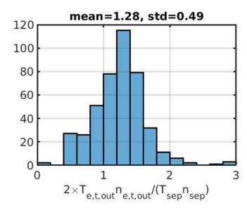
Figure 7. WEST C4–C5 database, B = 3.7 T,  $I_p = 0.5 \text{ MA}$ , LSN, D only,  $P_{\text{tot}} > 2$  MW. Histogram of the ratio  $\frac{2ne.t}{n_{e.t}T_{e.t}}$ .
