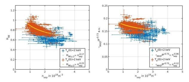
**Figure 5.** WEST C4–C5 L-mode database, B = 3.7 T,  $I_p = 0.5$  MA, LSN, D only,  $P_{\text{tot}} > 2$  MW. The confinement time is normalized to the H<sub>98y,2</sub> scaling law on the left and to the power degradation,  $P^{-0.73}$ , on the right. The normalized  $\tau_{MHD}$  is plotted versus the density at the separatrix measured by reflectometry,  $n_{\text{sep}}$ . The error bars represent the standard deviation measured during the plateaus over which the quantities are time averaged.
