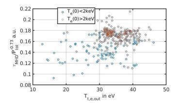
**Figure 17.** WEST C4 L-mode database, B = 3.7 T,  $I_p = 0.5$  MA, LSN, D only,  $P_{tot} > 2$  MW. The energy confinement time over its power degradation in arbitrary units:  $\tau_{MHD}/P_{tot}^{-0.73}$  is plotted against the outer target temperature measured by Langmuir probes.
