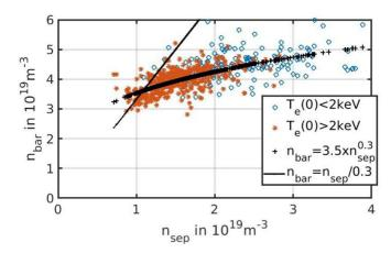
**Figure 10.** WEST C4–C5 L-mode database, B = 3.7 T,  $I_p = 0.5$  MA, LSN, D only,  $P_{\text{tot}} > 2$  MW. The plotted quantities are time averaged over the database plateaus. The line-averaged density from interferometry,  $n_{\text{bar}}$ , is plotted against the density at the separatrix,  $n_{\text{sep}}$ , measured by reflectometry. The plateaus over which the central electron temperature  $T_e(0)$  is below 2 keV are in blue, and in red where  $T_e(0) > 2$  keV.
