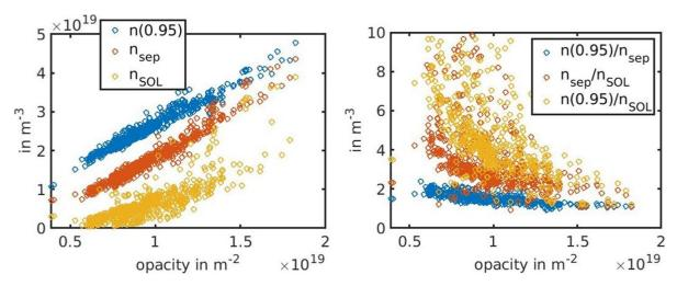
Figure 21. WEST C4–C5 L-mode database, B = 3.7 T,  $I_p = 0.5$  MA, LSN, D only,  $P_{tot} > 2$  MW. The densities are measured by reflectometry at 0.95, 1 and 1.05 of normalized poloidal flux for n(0.95),  $n_{sep}$  and  $n_{SOL}$ , respectively.
