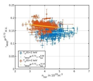
**Figure 4.** WEST C4–C5 L-mode database, B = 3.7 T,  $I_p = 0.5$  MA, D only, LSN,  $P_{\text{tot}} > 2$  MW. The error bars represent the standard deviation measured during the plateaus over which the quantities are time averaged. The confinement time is normalized to the power dependence of the WEST scaling law [2, 61]:  $P^{-0.73}$ .
