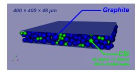
Figure 1 : DEM model of anode sample
