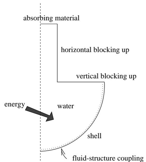
Figure 2: Geometrical model
