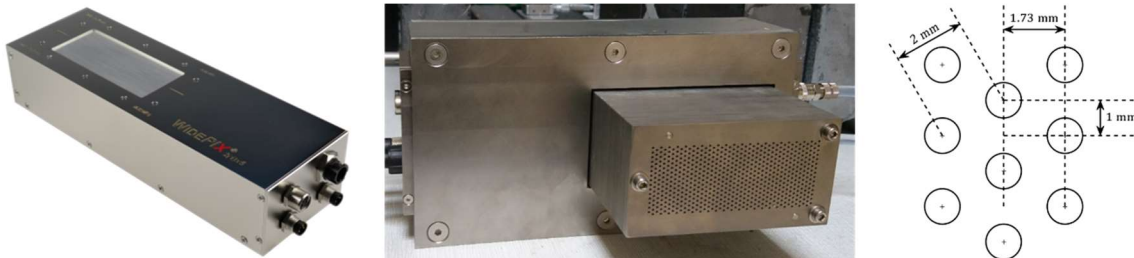
Figure 5: On the left: the WidePIX detector [4]; at the center: the WidePIX detector associated with the manufactured collimator; on the right: the pattern and dimensions of septa and holes defining the manufactured collimator.
