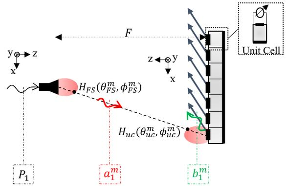
Fig. 1. Operating principle of the RIS in reflecting mode.
