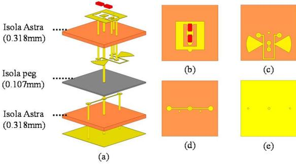
Fig. 2. The proposed 1-bit linearly-polarized unit-cell: (a) Schematic view, (b) radiating element, (c) biasing layer, (d) DC connection to the ground layer, and (e) ground plane.
