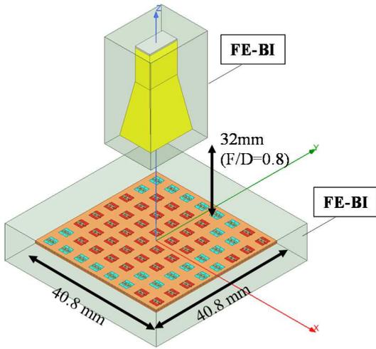
Fig. 7. The HFSS simulation setup of a RA of 8x8 unit cells illuminated in the middle by a standard 10dBi horn.
