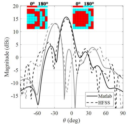
Fig. 8. The 2D gain pattern of the RA of 8x8 unit cells at 29GHz in the plane  $\phi=0^\circ$  for two steering angles  $-30^\circ$  and  $-10^\circ$ .
