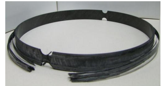
NOL ring after fatigue cycles
