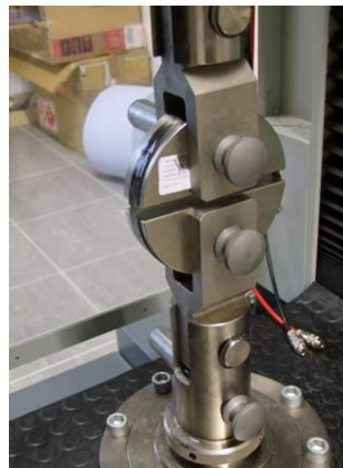
NOL ring installed on the testing machine
