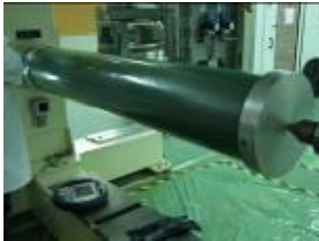
1. pre-preg carbon-expoxy with optical fibres laid on surface
