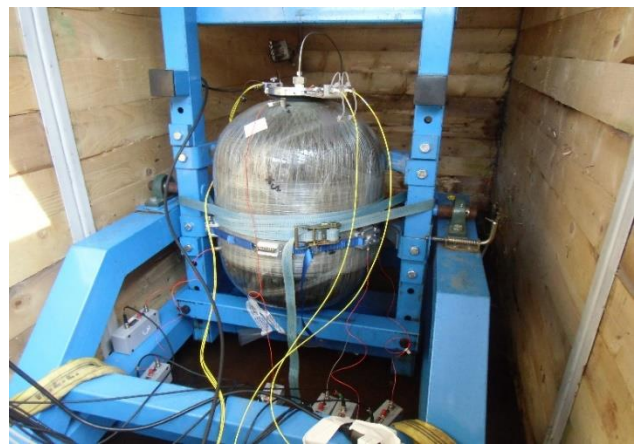
Composites Aquitaine™ burst test facility
