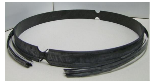
NOL ring after fatigue cycles
