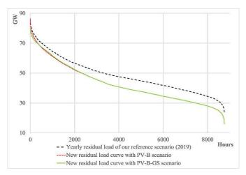
Figure 16: Changes in the load duration curve
