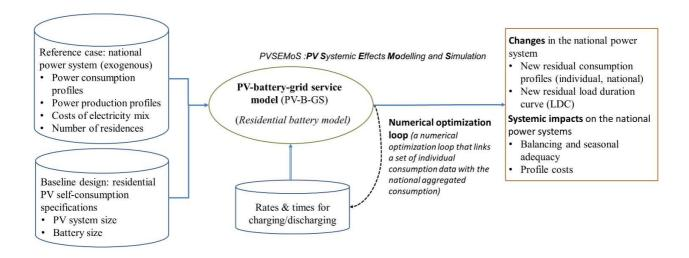
Figure 7: Logic flow diagram of the PV-B-GS (PV-battery-grid service) model
