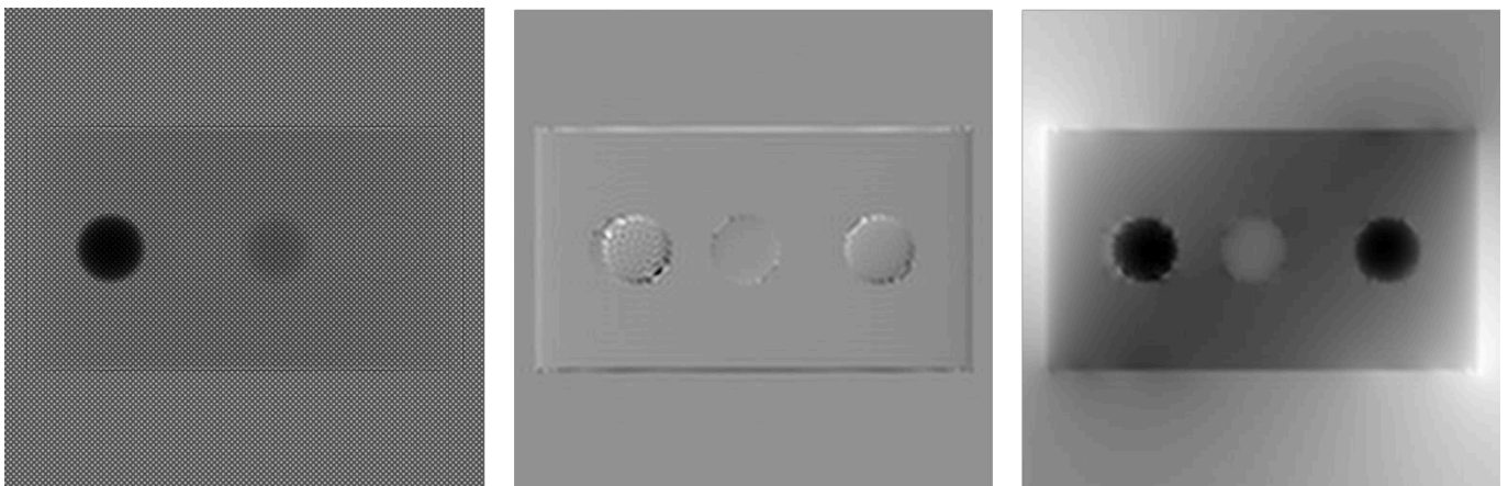
Figure 5: simulation result for one projection (a). The corresponding phase gradient (b) and phase image (c)
