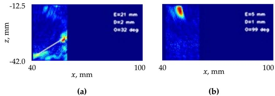
**Figure 10.** The DPS data set: the surface-breaking notch located 113 mm from the left edge, imaged from the notched side. MTFM images have been obtained with (a) intensity threshold = 125,  $D_m = -11$ , and (b) intensity threshold = 185,  $D_m = 15$ . Key as in Figure 7.
