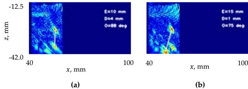
**Figure 7.** DPS data set: the buried notch located 113 mm from the left edge, imaged from the flat side. MTFM images have been obtained with intensity threshold = 185 and  $D_m$  = (a) 24; (b) 21. Key: E—notch extent, D—notch depth and O—notch orientation. The portion of the image to the left of the region of interest is cut off.
