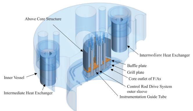
Fig. 5. Bird's eye view of CFD model.
