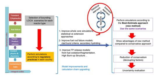
Fig. 4. R2CA methodology for best-estimate evaluation of releases during a LOCA transient.
