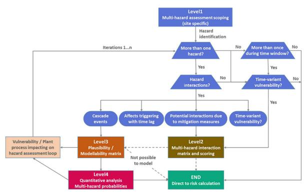
Fig. 3. The NARSIS MH framework scheme for scenarios to be used into multi-hazard PSA.
