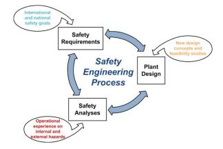
Fig. 7. Main elements of safety design and potential reasons to the changes.
