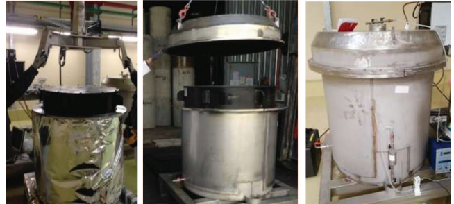
Fig. 17. 870 L FI setup in airtight enclosure (middle) and closed airflow circuit for accumulation data acquisition (right).
