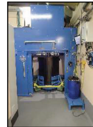
Fig. 21. Packaging of unused sealed sources.
