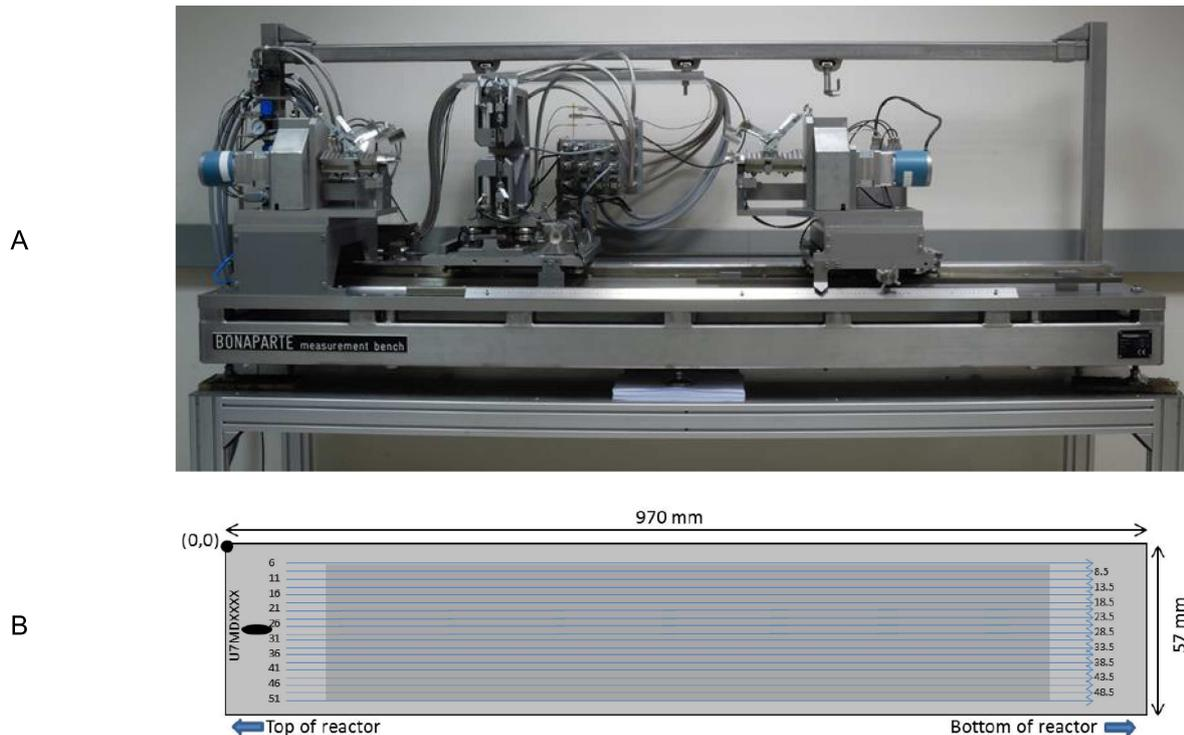
**Fig. 5.** (A) The BONAPARTE measuring device. (B) Coordinate system adopted for the BONAPARTE measurement results for a typical FUTURE plate.
