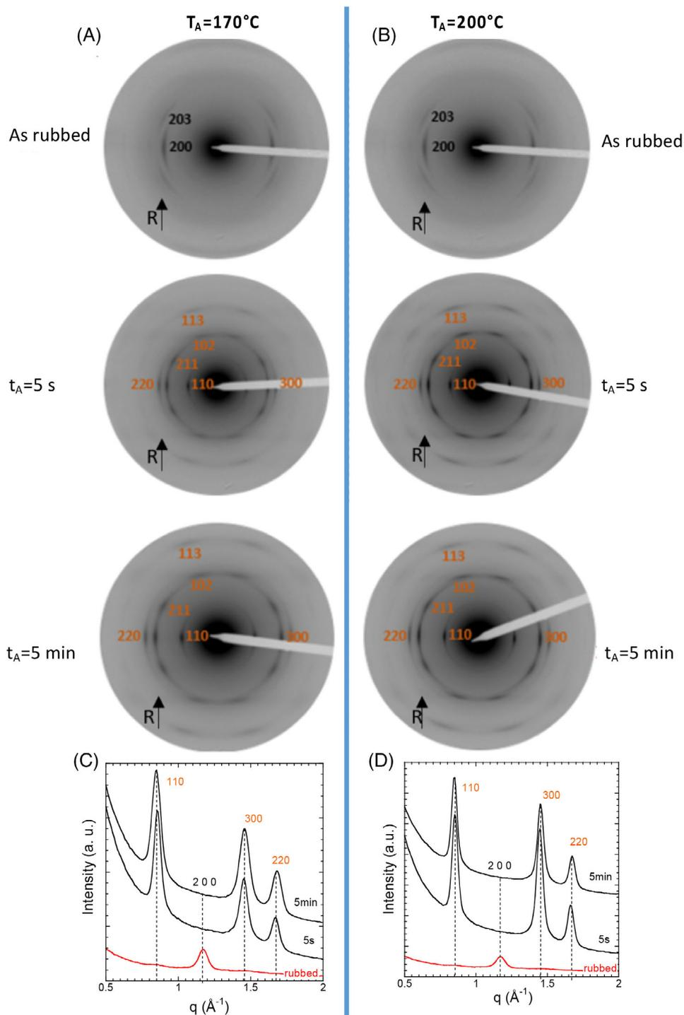
**FIGURE 6** Impact of annealing time ( $t_A$ ) on the electron diffraction patterns of rubbed PLLA/PDLA equimolar blend films ( $T_R = 100^\circ\text{C}$ , 50 nm). The rubbing direction is vertical. The indices for the reflections of the PLLA and PDLA homocrystals are in black whereas the reflections of the SC-PLA phase are noted in orange. Equatorial section profiles of the ED patterns versus annealing time for  $T_A = 170^\circ\text{C}$  (B) and  $T_A = 200^\circ\text{C}$  (C).
