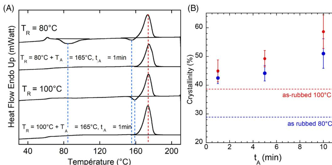
**FIGURE 3** (A) DSC traces of the first annealing scan of PLLA thin films rubbed at 80 and 100°C. Cold crystallization exotherms are highlighted in blue whereas melting endotherms are shown in red. Evolution of the crystallinity (B) extracted from the melting enthalpies for PLLA films rubbed at 80°C (blue) and 100°C (red) and annealed at 165°C for different times.
