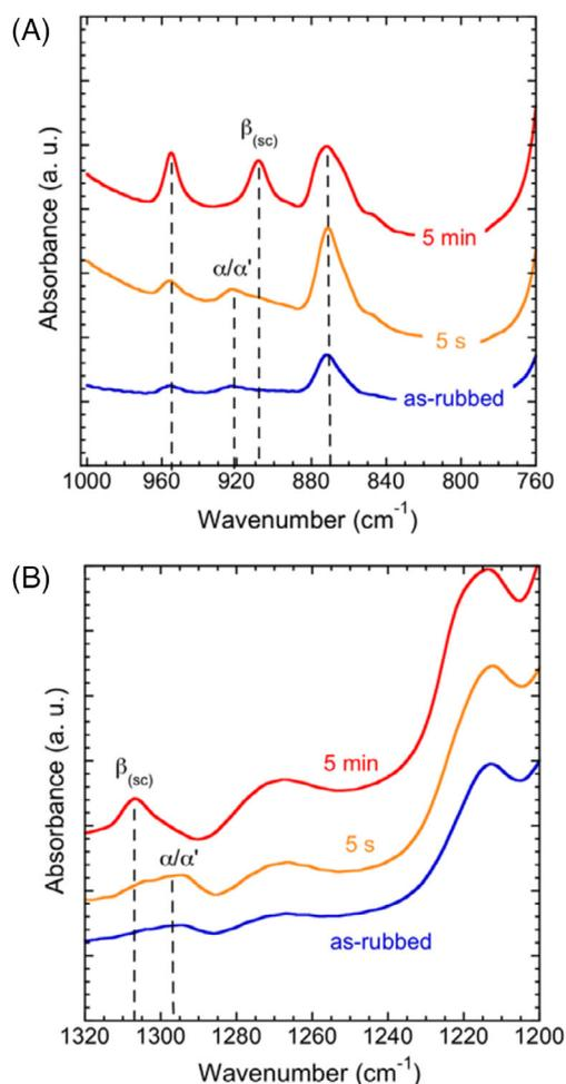
**FIGURE 7** Evolution of the FTIR spectra of rubbed PLLA/PDLA (1:1) blend films rubbed at  $T_R = 100^\circ\text{C}$  as function of the annealing time  $t_A$  at  $T_A = 200^\circ\text{C}$ . (A) 800–1000  $\text{cm}^{-1}$  range and (B) 1200–1320  $\text{cm}^{-1}$ . For clarity, spectra were shifted along the ordinate axis.
