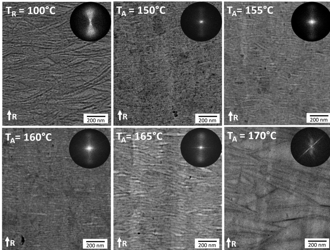
**Figure 2:** Evolution of the lamellar morphology in rubbed PLLA films ( $T_R=100^\circ\text{C}$ ) as a function of the annealing temperature  $T_A$  (the annealing time was 5 min). The insets show the FFT of the BF images. The rubbing direction is vertical.
