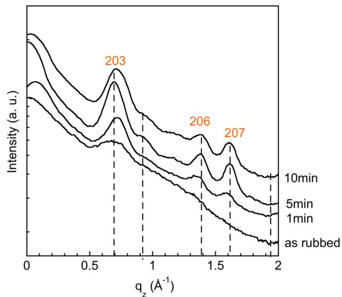
**Figure S3.** Section profile along  $q_z$  ( $h=2$ ) in the ED pattern of a PLLA film oriented at  $T_R=100^\circ\text{C}$  and annealed at  $165^\circ\text{C}$  for different annealing times. Indexation of the reflections is according to the  $\alpha$  form of PLLA
