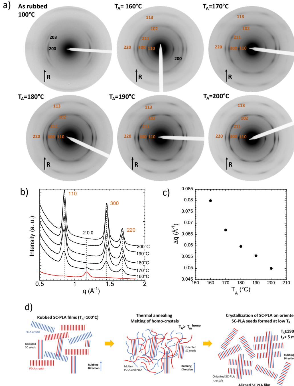
**Figure 5.** a) Evolution of the ED patterns of rubbed PLLA/PDLA equimolar blend films ( $T_R = 100^\circ\text{C}$ ) as a function of the annealing temperature  $T_A$  (duration of annealing of 5 min). The rubbing direction is vertical. The indices for the reflections of the PLLA and PDLA homo-crystals are in black whereas the reflections of the SC-PLA phase are noted in orange. b) Equatorial section profiles of the ED patterns *versus* annealing temperature ( $T_A$ ). c) FWHM of the 3 0 0
