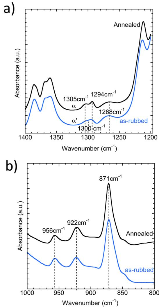
**Figure S2.** FTIR spectra of a rubbed PLLA film (150nm,  $T_R=100^\circ\text{C}$ ) (blue) and after thermal annealing (5 min,  $165^\circ\text{C}$ ). a) spectral range  $1200\text{-}1400\text{ cm}^{-1}$  and b) spectral range  $800\text{-}1000\text{ cm}^{-1}$
