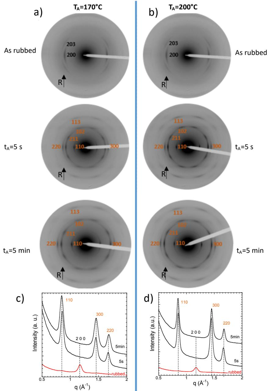
**Figure 6.** Impact of annealing time ( $t_A$ ) on the electron diffraction patterns of rubbed PLLA/PDLA equimolar blend films ( $T_R=100^\circ\text{C}$ , 50nm). The rubbing direction is vertical. The indices for the reflections of the PLLA and PDLA homocrystals are in black whereas the
