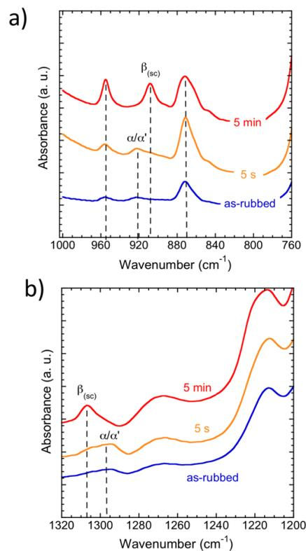
**Figure 7.** Evolution of the FTIR spectra of rubbed PLLA/PDLA (1:1) blend films rubbed at  $T_R=100^\circ\text{C}$  as function of the annealing time  $t_A$  at  $T_A=200^\circ\text{C}$ . a) 800-1000  $\text{cm}^{-1}$  range and b) 1200-1320  $\text{cm}^{-1}$ . For clarity, spectra were shifted along the ordinate axis.
