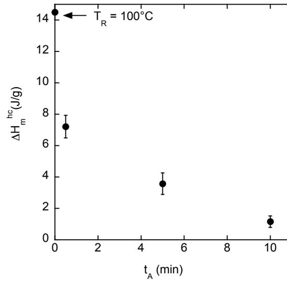
**Figure S4.** Evolution of the melting enthalpy  $\Delta H_m^{\text{homo}}$  of the PLA homocrystals in a rubbed PLLA/PDLA (1:1) film after thermal annealing at  $165^\circ\text{C}$  for different annealing times  $t_A$ .  $t_A=0$  corresponds to the as-rubbed film without annealing.
