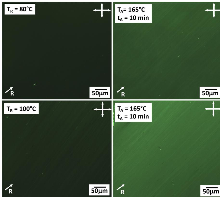
**Figure S1.** POM images under crossed polarizers of oriented PLLA thin films rubbed at 80°C and 100°C and after thermal annealing à 165°C for 10 min. Note the stronger birefringence obtained for the films rubbed initially at 100°C. The rubbing direction is indicated by an arrow.
