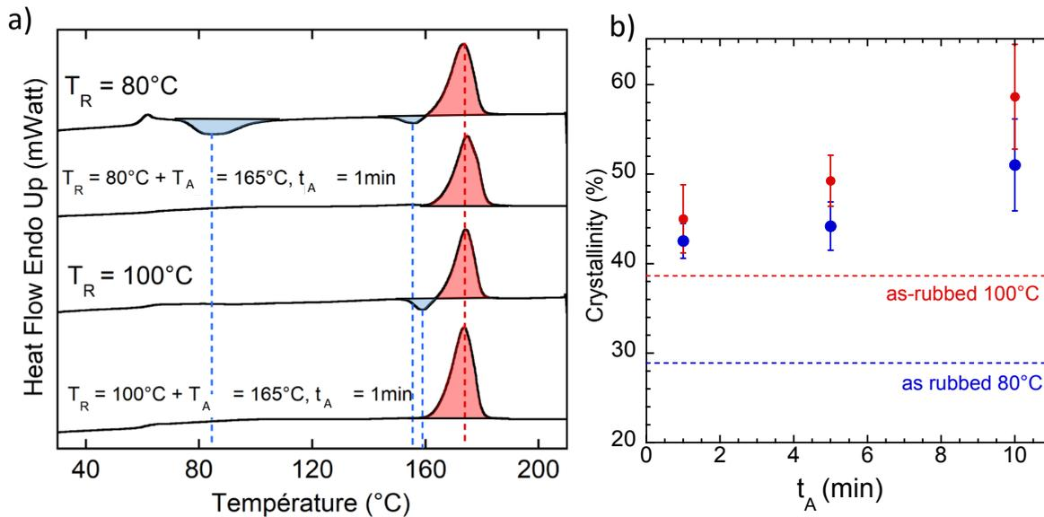
**Figure 3:** a) DSC traces of the first annealing scan of PLLA thin films rubbed at  $80^\circ\text{C}$  and  $100^\circ\text{C}$ . Cold crystallization exotherms are highlighted in blue whereas melting endotherms are shown in red. Evolution of the crystallinity (b) extracted from the melting enthalpies for PLLA films rubbed at  $80^\circ\text{C}$  (blue) and  $100^\circ\text{C}$  (red) and annealed at  $165^\circ\text{C}$  for different times.
