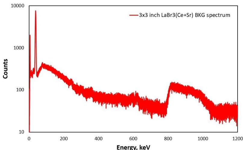
**Figure 4:** Background radiation spectrum measured on a 3x3 inch LaBr<sub>3</sub>(Ce+Sr) detector.
