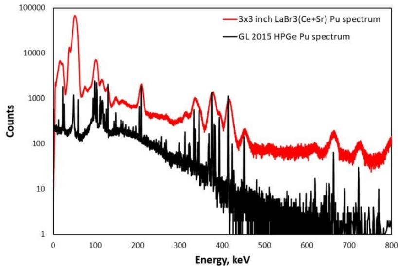
**Figure 3:** Spectrometric performance comparison of 3x3 inch LaBr<sub>3</sub>(Ce+Sr) and GL 2015 HPGe detectors.
