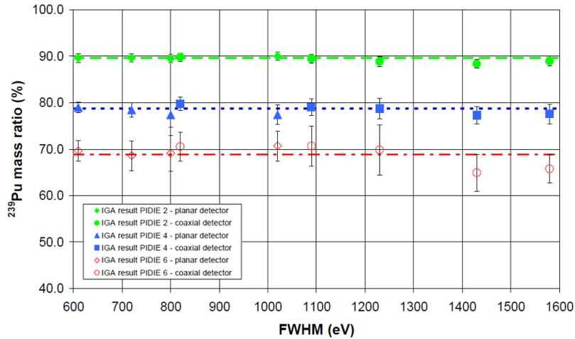
**Figure 2:** Impact of the detector energy resolution on the IGA code performance with Pu samples of different isotopic composition [37].
