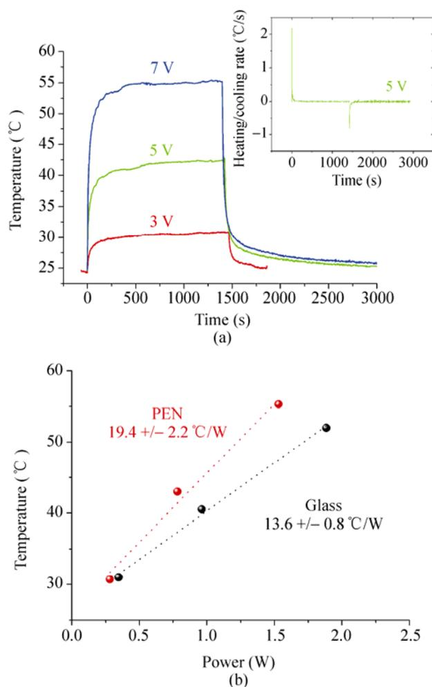
**Figure 4** (a) Heating experiments showing temperature as a function of time for a 35  $\Omega/\text{sq}$ . TTFH on a 125  $\mu\text{m}$  PEN substrate at different applied voltages. Inset: derivative of the temperature vs. time at 5 V applied bias. (b) Input power as a function of the steady state temperature on PEN and glass substrates
