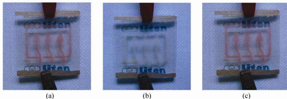
**Figure 5** Thermochromic display made with Ag-NW based TTFH ( $89\%$  T550 nm– $82\text{ }\Omega/\text{sq}$ .); (a) at room temperature; (b) after applying 12 V; (c) after returning to room temperature
