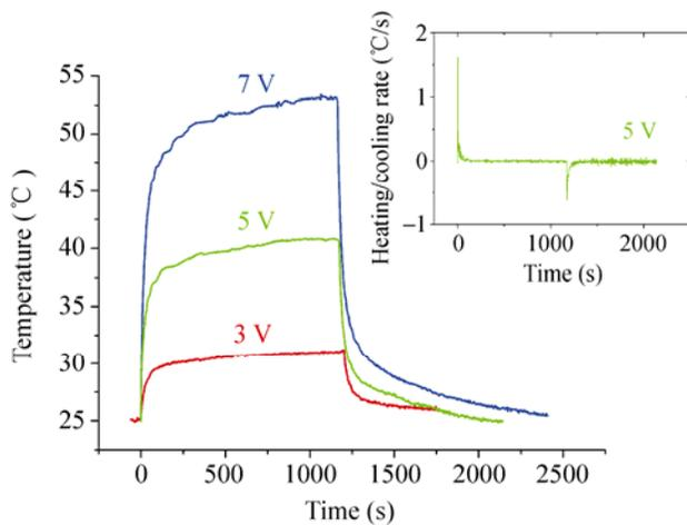
**Figure 2** Heating experiments showing temperature as a function of time for a 33 Ω/sq. TTFH on glass at different applied voltages (20 min duration). Insert: derivative of the temperature vs. time at 5 V applied bias
