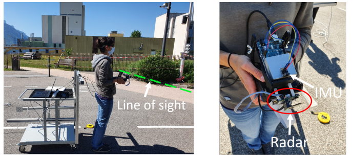
Fig. 9. Experimental setup including MIMO radar and IMU
