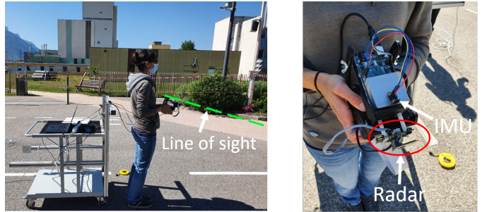
Fig. 9. Experimental setup including MIMO radar and IMU
