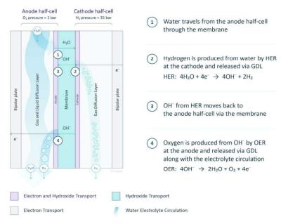
Figure 1: schematic AEM water electrolysis
