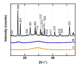
Fig. 5. XRD spectra for materials A to E annealed at 400°C. B and D spectra match A and C spectra respectively (not reported). E material remains perfectly amorphous after annealing (i.e. no crystalline patterns). Peaks detected in the other samples are attributed to Sb<sub>2</sub>Se<sub>3</sub> crystalline phase (orthorhombic Pnma (62) space group of ICDD database).
