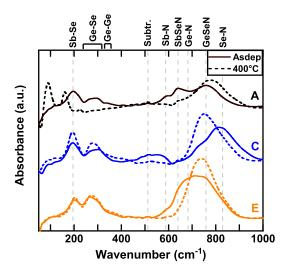
Fig. 4. FTIR spectra for A, C and E samples as-deposited and annealed at 400°C. A material is degraded by the 400°C annealing, as show the Sb-Se and Ge-Se features. Considering the N-related bonds, annealing tends to reduce the number of different features favouring stable Ge-N or Ge-Se-N bonds [23].
