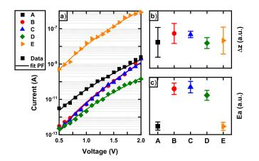
Fig. 10. a) Median I-V characteristics with Poole-Frenkel fits, b) Intertrap distance calculated with eq. (1) and, c Activation energy  $E_a$  extracpolated from eq. (2).
