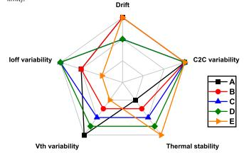
Fig. 15. Radar graph showing the different electrical performances studied in  $Ge_x(SbSe)_{1-x}N$  OTS devices. Best compromise should be found in layers with intermediate Ge content i.e. C and D compositions.
