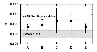
Fig. 14. Drift coefficient  $\alpha$  measured thanks to eq. (5). We can observe that C and D materials present the highest drift, leading to an increase of 0.25 V (i.e. about + 6%) after 10 years. Some devices present an  $\alpha$  value too low to be measured correctly (grey banner, under detection limit).
