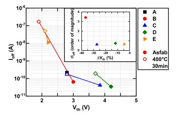
Fig. 9. I<sub>off</sub> as a function of V<sub>th</sub> for Ge<sub>x</sub>(SbSe)<sub>1-x</sub>N devices, extracted from Fig. 7 and Fig. 8, before and after annealing. Inset: variation of the order of magnitude of I<sub>off</sub> (rI<sub>off</sub>), calculated as the log<sub>10</sub> of the ratio between the value after and before annealing, as a function of the V<sub>th</sub> variation in % before and after annealing.
