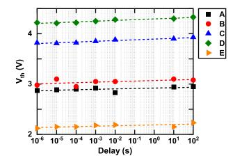
Fig. 13.  $V_{th}$  measured after 1 µs, 10 µs, 100 µs,1 ms, 10 ms, 10 s and 100 s delay. Dashed lines represent the fitting curves obtained using equation eq. (5).
