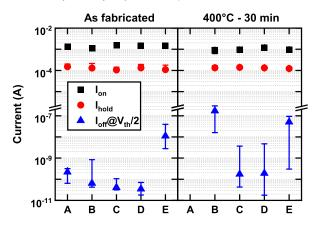
Fig. 8.  $I_{on}$ ,  $I_{hold}$  and  $I_{off}$  measured for the Ge<sub>x</sub>(SbSe)<sub>1-x</sub>N OTS devices before and after annealing at 400°C. The parameters are acquired after 1000 cycles. Data for material A are not reported after annealing due to devices failure related to the layer crystallization (Fig. 5).
