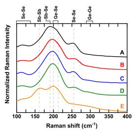
Fig. 1. Raman spectra of as-deposited materials. Main feature at 200 cm<sup>-1</sup> is the result of the convolution of Sb-Se (at 190 cm<sup>-1</sup>) and Ge-Se vibrations (at 200 and 210 cm<sup>-1</sup>). Increasing Ge content from composition A to E, we observe a decrease of Se-Se mode (at 245-265 cm<sup>-1</sup>) and an increase of Sb-Sb mode (at 160 cm<sup>-1</sup>) [10]–[12].
