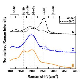
Fig. 2. Raman spectra for A, C and E samples as-deposited and after annealing at 400°C. Results from layers B and D are not reported for sake of clarity, being the results obtained for B close to A, and for D close to C. A strong Se segregation is observed in A leading to important material degradation. Annealing reduces Se segregation in C by slightly increasing the Ge-Se content. Material E stays stable after annealing.
