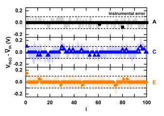
Fig. 12.  $V_{th}$  cycle-to-cycle variation measured along 100 switching operations, after 10<sup>4</sup> cycles. The  $V_{th}$  variation (y-axis) is calculated as the difference between  $V_{th}$  measured at i-th cycle ( $V_{th}(i)$ ) and the mean value of  $V_{th}$  calculated for the 100 consecutive cycles ( $\overline{V_{th}}$ ).
