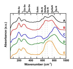
Fig. 3. FTIR spectra of as-deposited materials. Main features are identified to be related to Sb-Se at 201 cm<sup>-1</sup> [19], Ge-Se at 250- $300 \text{ cm}^{-1}$  [16], [19], [20] and N-related bonds above 590 cm<sup>-1</sup> [17], [21]–[24].
