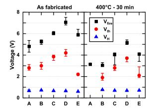
Fig. 7.  $V_{fire}$ ,  $V_{th}$ ,  $V_{H}$  measured for all  $Ge_x(SbSe)_{1-x}N$  OTS devices before and after annealing at 400°C. The values of  $V_{th}$  and  $V_{H}$  are collected after 1000 cycles (to confirm the device reliable functionality and stable cycle-to-cycle parameters).
