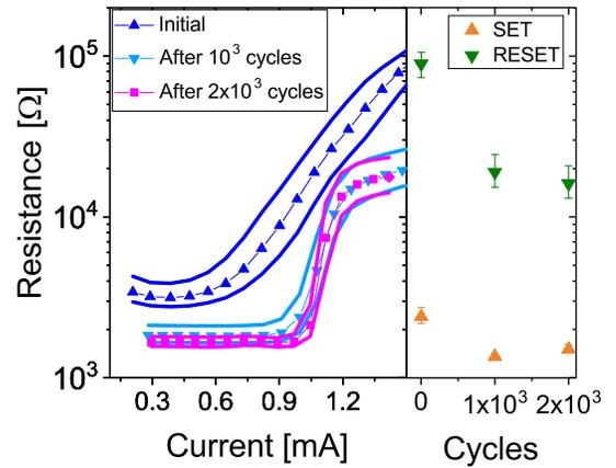
**Fig. 8.** Left: R-I characteristic at the beginning of the devices life and after endurance for TiTe/GST. Right: 4 kb TiTe/GST SET and RESET resistances evolution along cycles performed with pulses of 10  $\mu$ s to accelerate and evidence the evolution.
