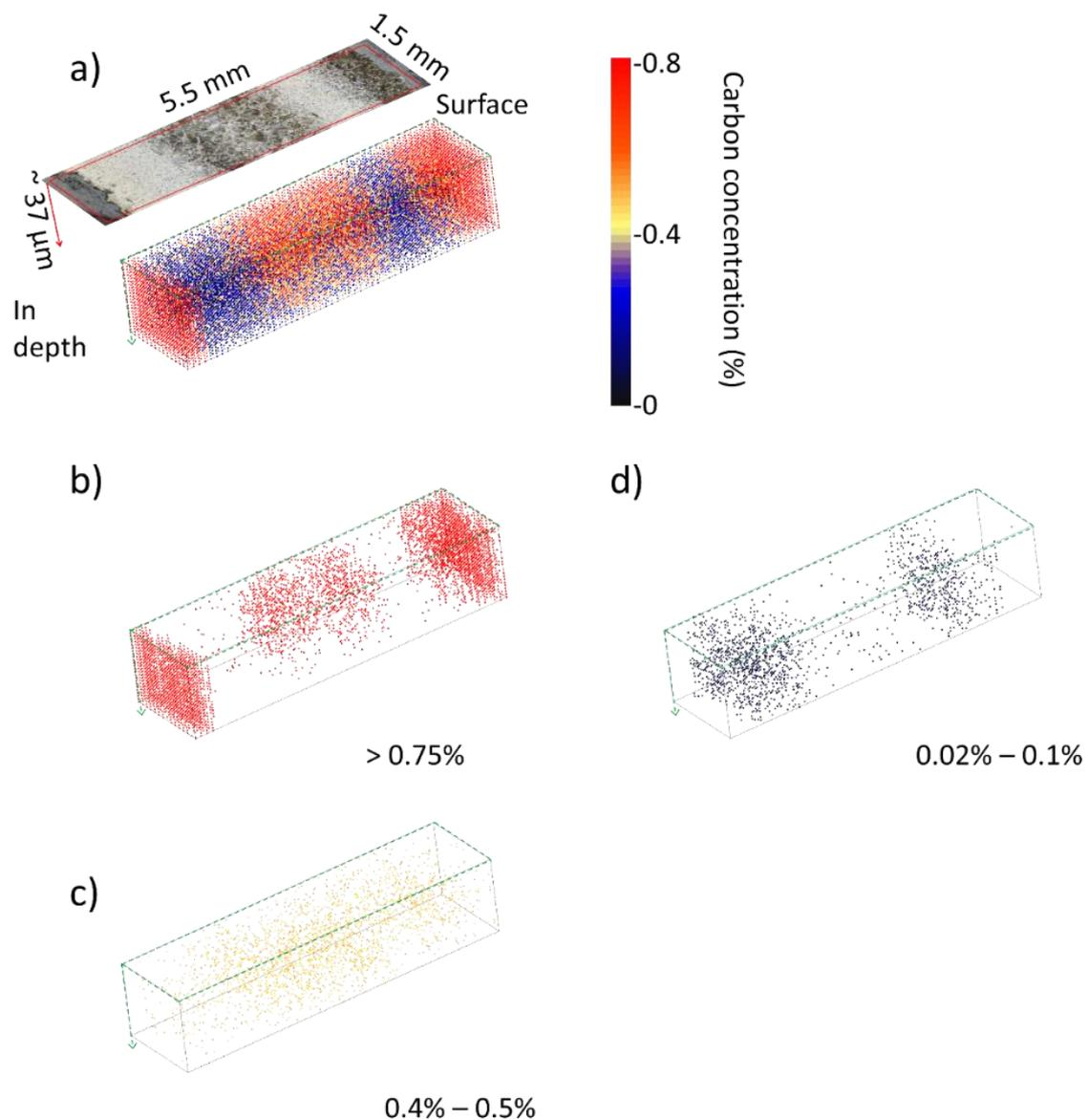
Fig. 8 Micro-LIBS volume analyses on the archaeological piece CL13286b with equilibrium state with 3D representation in different carbon concentration range: a)  $>0.02\%$ ; b)  $>0.75\%$ ; c)  $0.4\% - 0.5\%$ ; d)  $0.02\% - 0.1\%$ . The surface is marked with green dot-line, and the arrow indicated the depth direction.
