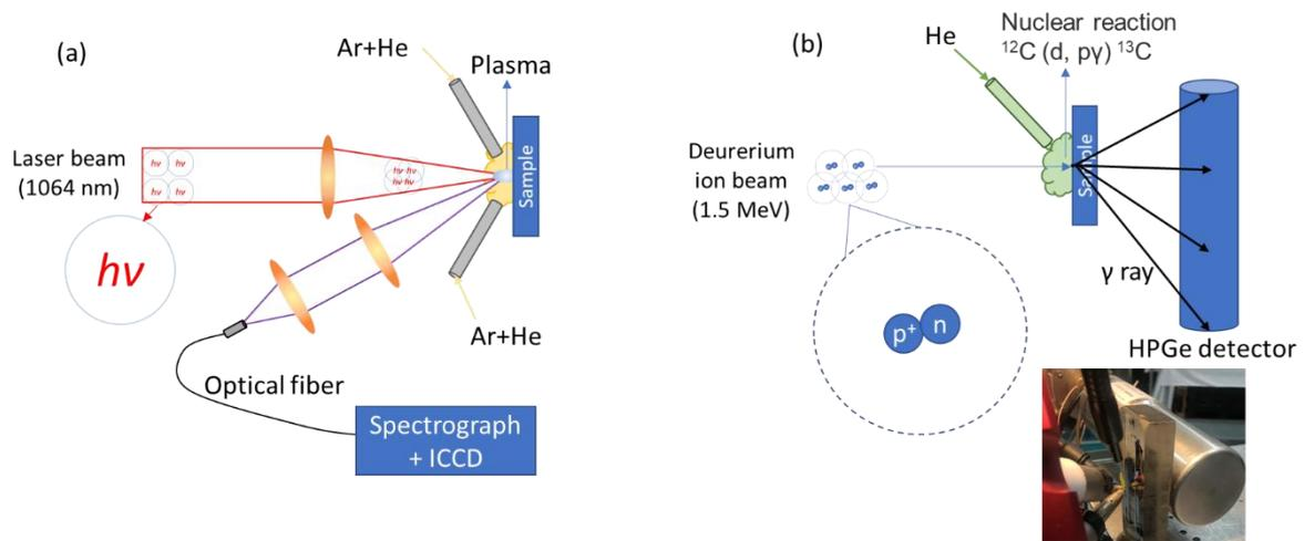
Fig. 2 Experimental setup: (a) LIBS setup; (b) IBA of deuterium setup with the insert photography of the setup in the laboratory.
