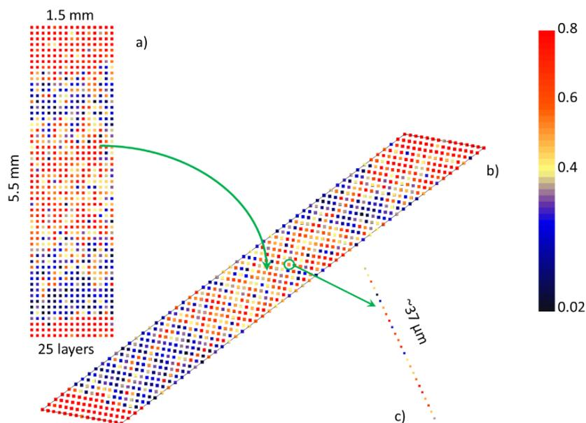
Fig. 7 Micro-LIBS on the archaeological piece CL13286b (CM16, US6016) in-depth into different layers, for each layer, the carbon concentration is calculated by the averaged of ten laser shots. The top view (a) and 3D view (b) of carbon concentration distribution cube with the proportional dimension of the real size; c) stratigraphy of one point in the carbon concentration distribution cube.
