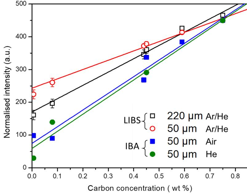
Fig. 4 Calibration curves of macro-LIBS under He/Ar atmosphere with 220  $\mu\text{m}$  of averaged 230 laser shots at one spot, micro-LIBS with 50  $\mu\text{m}$  of averaged 230 laser shots at one spot over nine spots, and deuterons ions beams in different gas environment.
