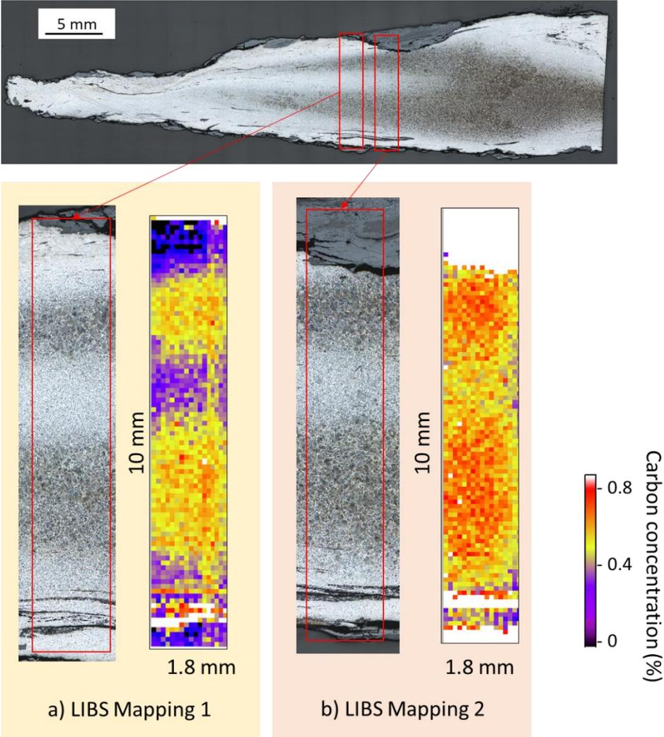
Fig. 6 Two micro-LIBS mapping images on the archaeological piece CL12247-3 (CM14, US3077) with Widmanstätten structure
