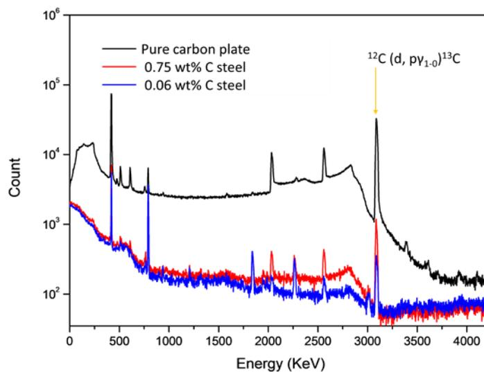
Fig. 3 Gamma spectra from pure carbon sample and two of reference sample excited by deuterium ion beam in He. The yellow arrow shows the gamma peak from carbon in reaction  $^{12}\text{C} (d, p\gamma_{1-0})^{13}\text{C}$
