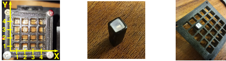
Figure 4: Left: the grid fixed on the holder of the H11934 PMT; Center: the plastic scintillator piece inserted in a holder covered with reflective foil; Right: the PS holder slides through each hole in the grid ensuring that the PS touches the PMT window.
