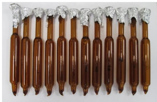
Fig. 14. Different bulbs with various components of the temperature sensing cable inside, after irradiation 3 at a dose of 1.8 MGy.
