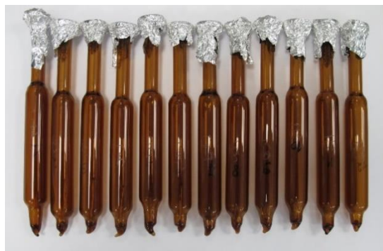
Fig. 14. Different bulbs with various components of the temperature sensing cable inside, after irradiation 3 at a dose of 1.8 MGy.
