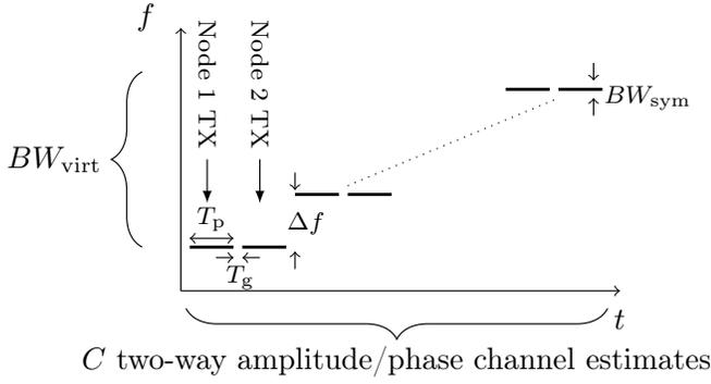
Fig. 1. Multi-channel ranging signaling process for  $C$  sequentially aggregated narrowband ( $BW_{\text{synt}}$ ) channels. The  $C$  channels form a virtual bandwidth equal to  $BW_{\text{virt}} = (C - 1)\Delta f$ .
